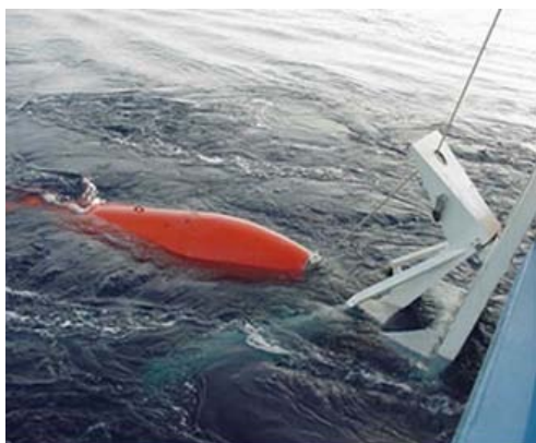
EdgeTech 4400-SAS Side Scan Sonar on Hugin 1000
